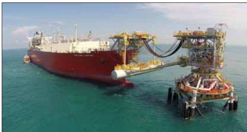
▲ PGN FSRU Lampung is Indonesia's latest floating regas terminal and the first to use a tower yoke mooring system.
